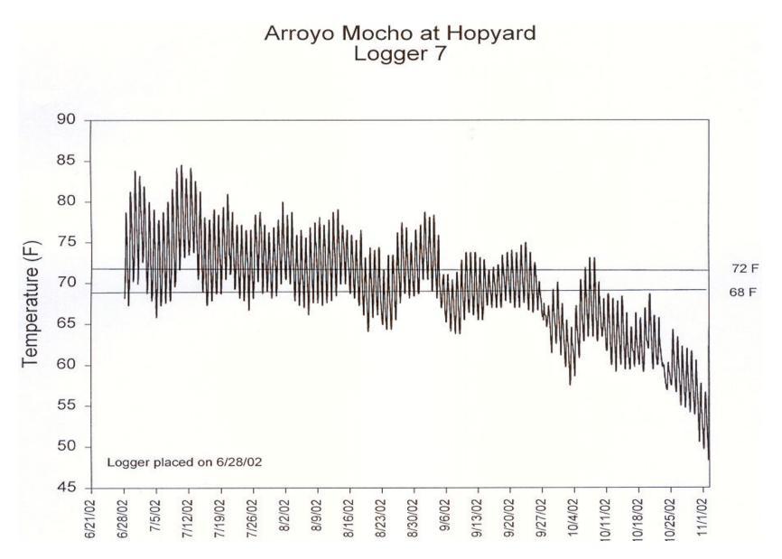
Figure 10. Hourly water temperatures measured at Arroyo Mocho at Hopyard (2002).
